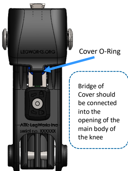
Fig. 23 All-Terrain Knee Cover Release
