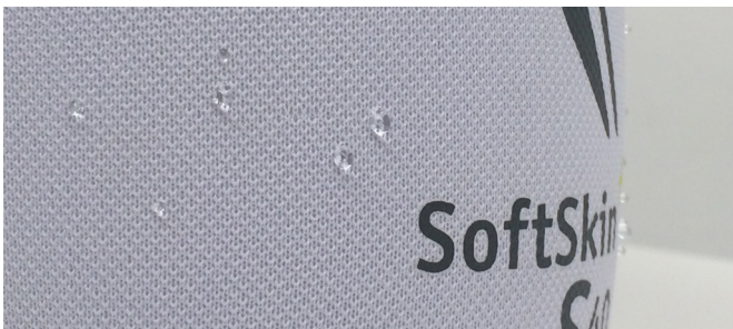
5. With successful activation of the micro-pores, water drops will leak on the outside.
