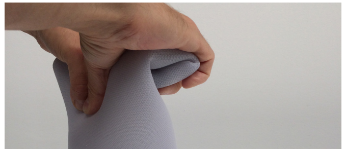
4. Fill the liner half (maximum) with water. Roll the upper end to close the liner until pressure occurs on the trapped water.
